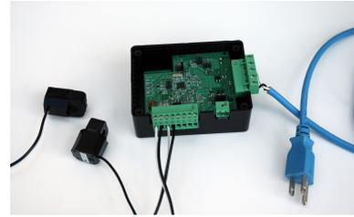
Figure 2: Wireless Three-Phase Circuit-Panel Meter
