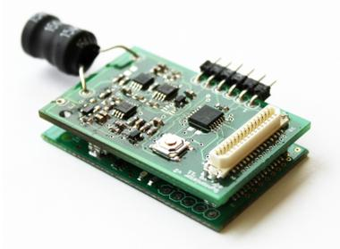
**Figure 5: EMF event detector stacked on Fire-Fly3 sensor node.**
