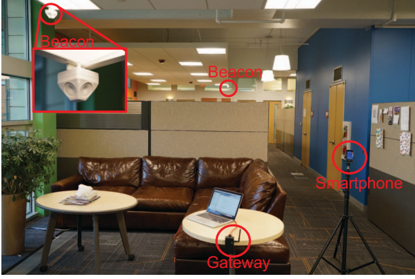
Figure 8: Experimental setup for data collection, with beacons, smartphone and gateway.
